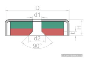
CSF-25 Ferrite pot magnet Ø 25 mm with countersunk hole Weight: 16 g
