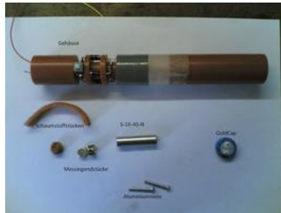
All the individual parts before the assembly. The spool received already a protective finish and is masked.
