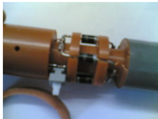
All the individual parts before the assembly. The spool received already a protective finish and is masked.
